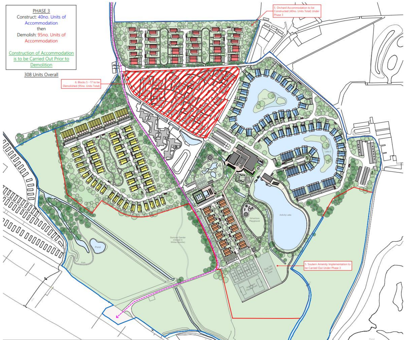
Figure 4.4: Indicative Construction Phasing Plan 03
