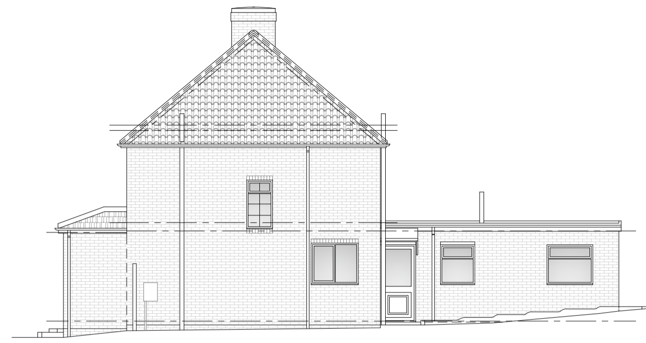
2 SIDE ELEVATION Scale 1:100
