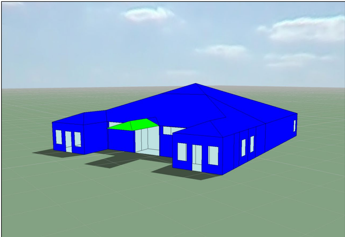
3D Model representation of the building in the SBEM calculation software (IES Virtual Environment). Geometry simplifications are made where appropriate.
