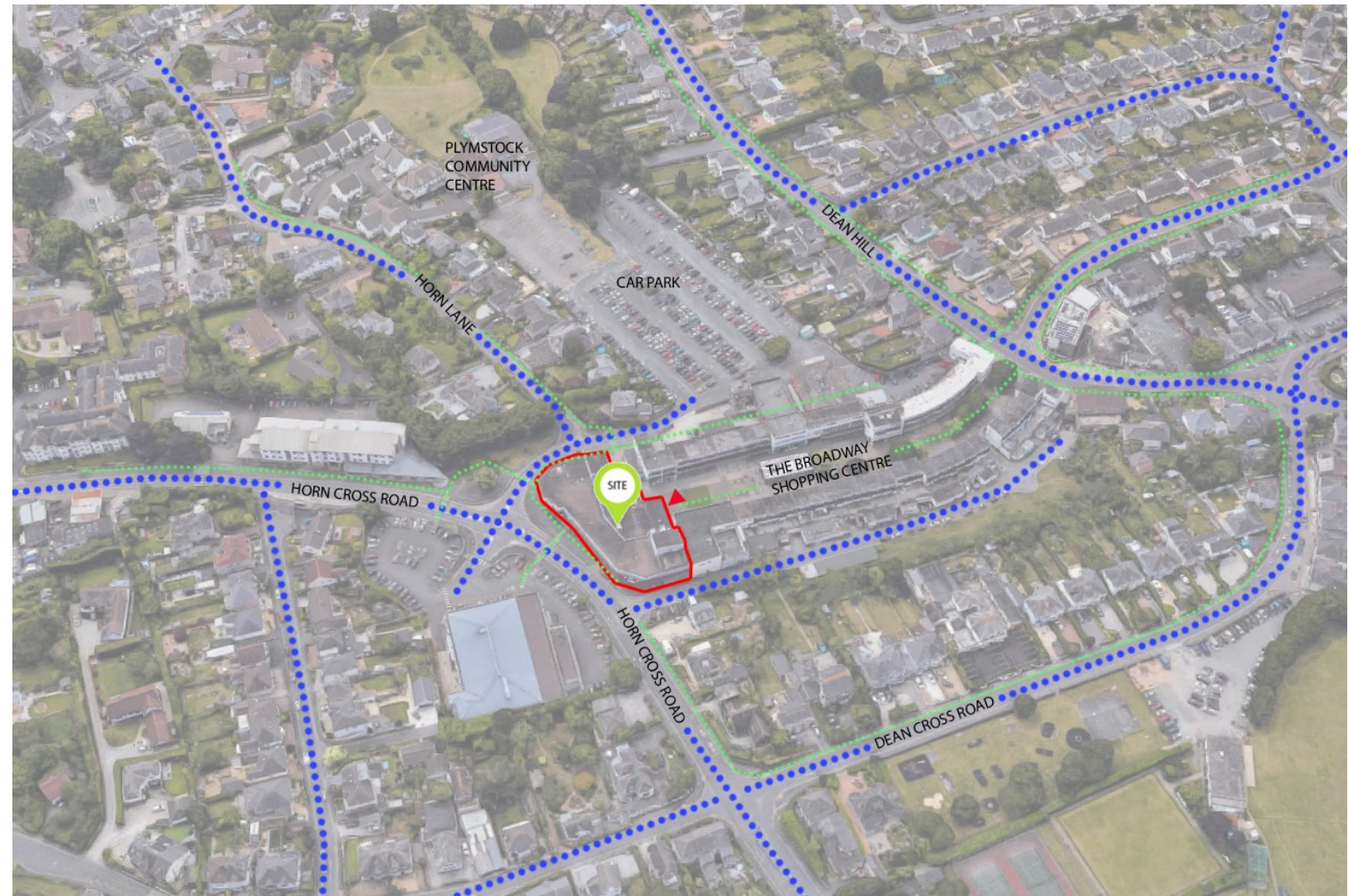
Pedestrian and Vehicle Routes Diagram – Blue dotted = Vehicle Routes, Green dotted = Pedestrian Routes
