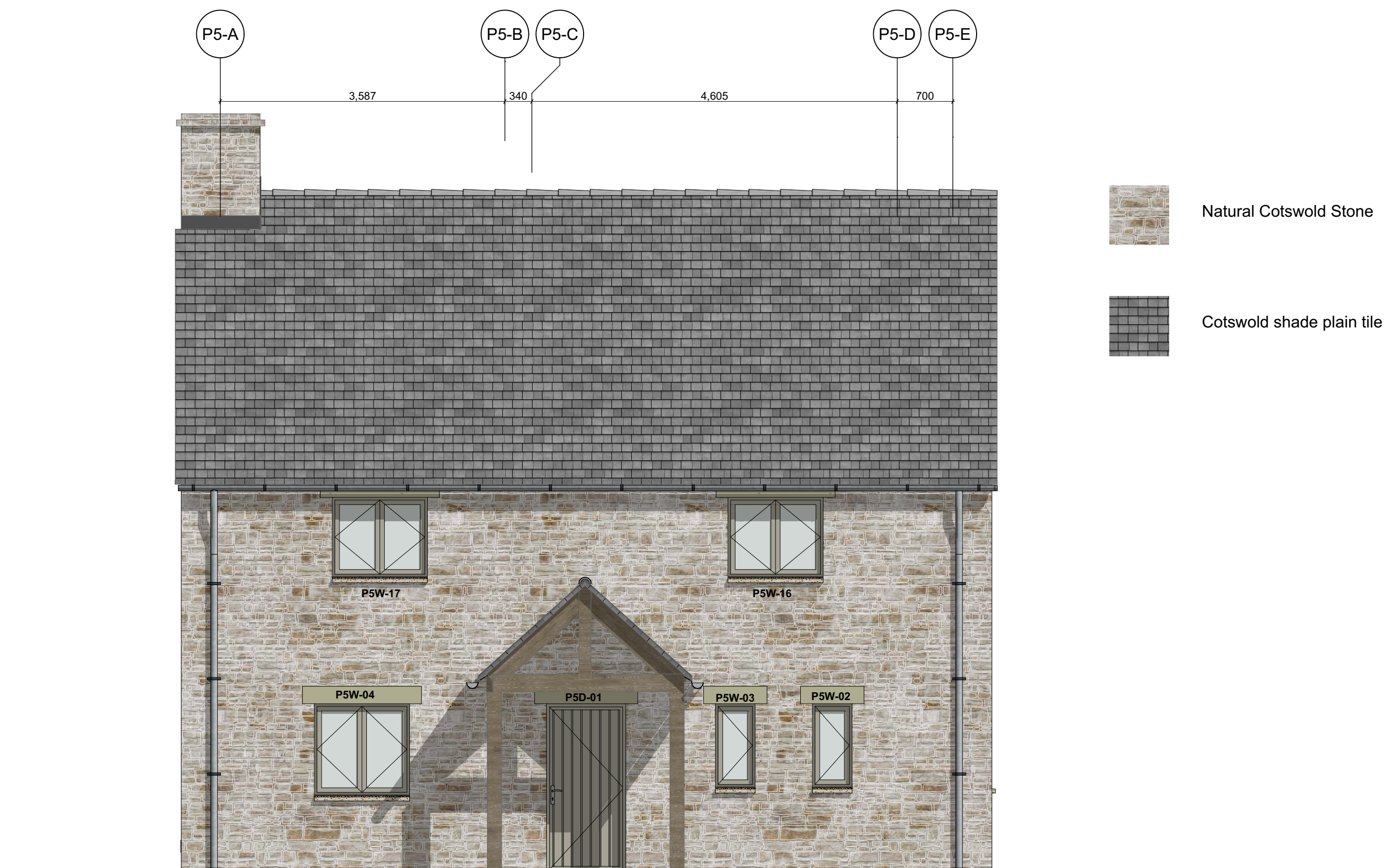
HF5 - West Elevation 1:50
