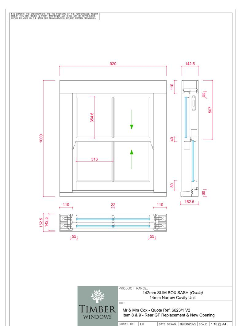
ALL MEASUREMENTS ARE FINISHED DIMENSIONS IN MM. DO NOT SCALE DRAWING!
