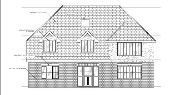
PROPOSED ELEVATION - FRONT (SCALE 1:100)
