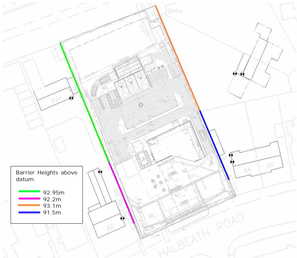
Figure A6.5 – Barrier heights used in the Cadna-A environmental noise model
