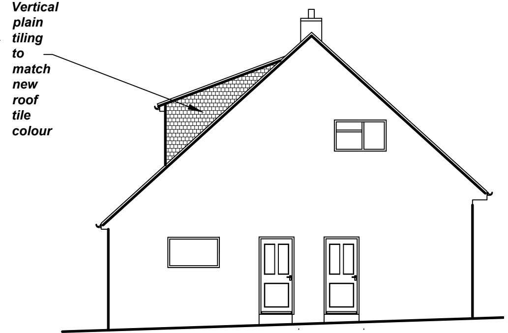
PROPOSED SOUTH EAST ELEVATION Scale 1:100
