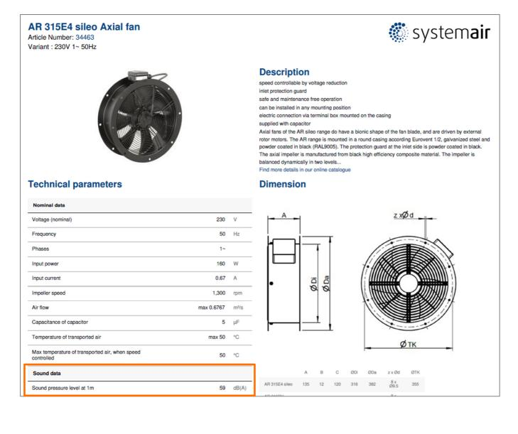
Note that only sound pressure level at 1m is available for this fan, and only in dB(A) terms, ie. not octave band (frequency band) information. We describe how we deal with this later.
