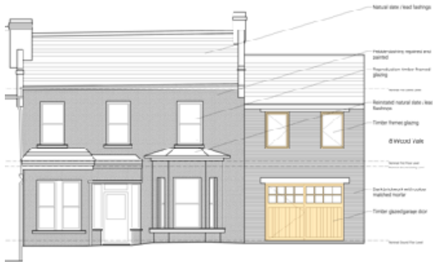
Front elevation proposed showing garage-style fenestration
