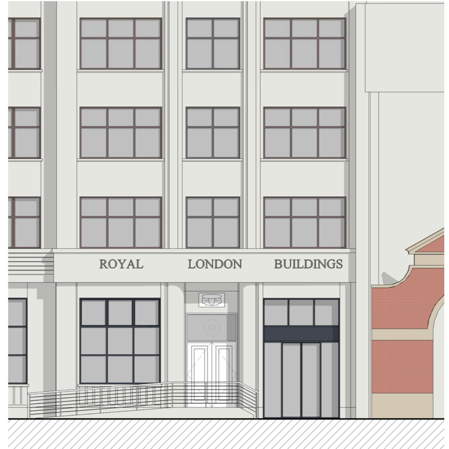
▲ Proposed new entrance sliding doors to the office lobby, with frames and proportion to match adjacent elements
