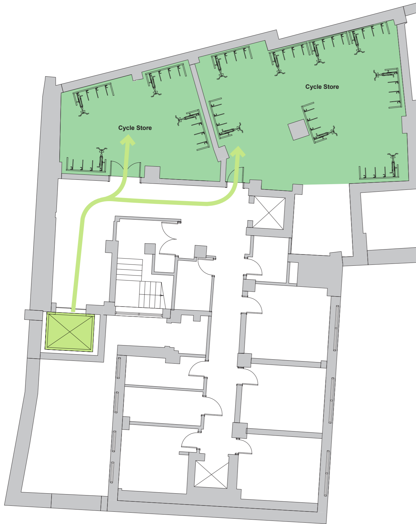
▲ Cyclists' access routes to the Basement cycle stores
