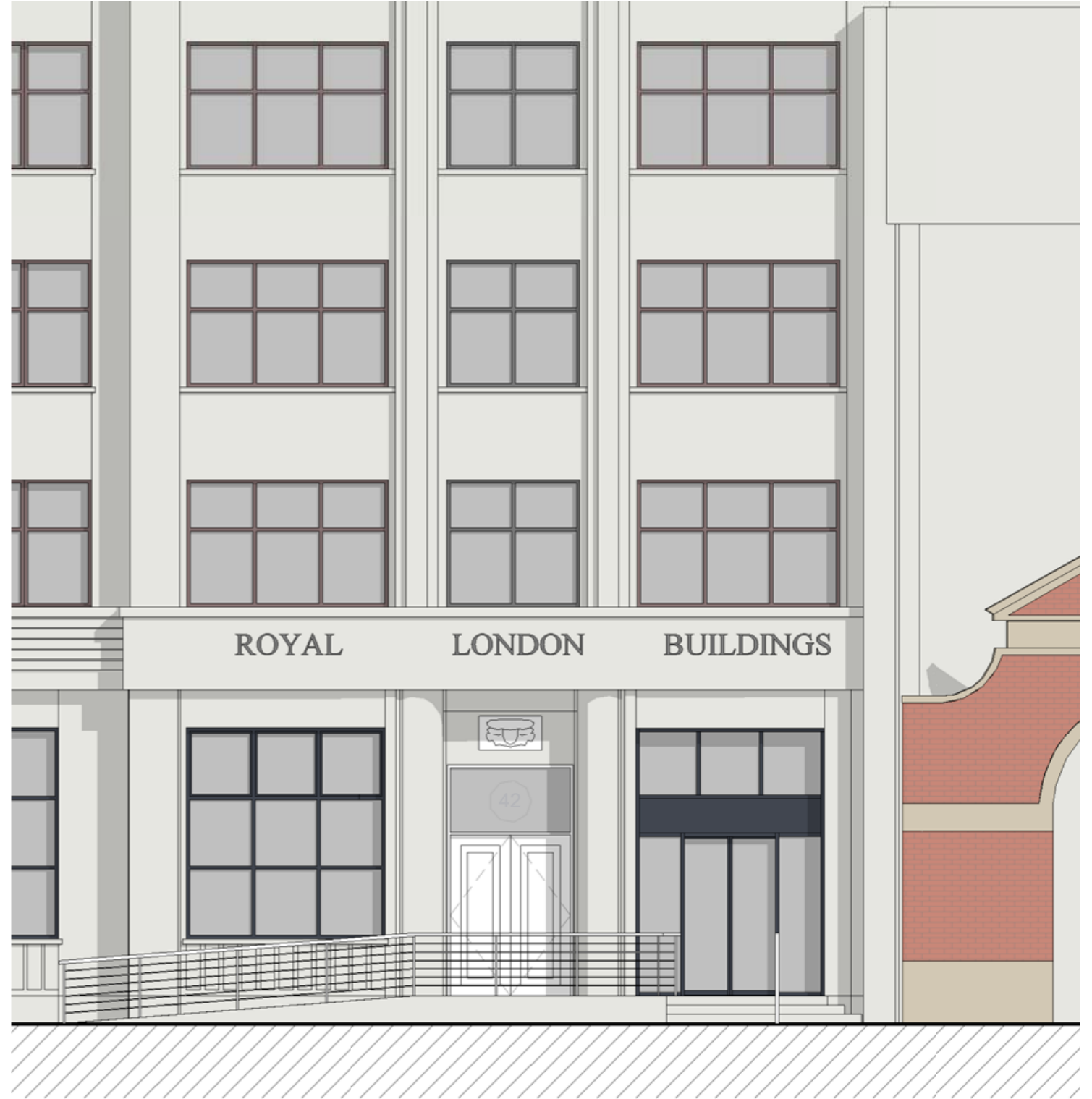
▲ Proposed new entrance sliding doors and steps to the office lobby, with frames and proportion to match adjacent elements
