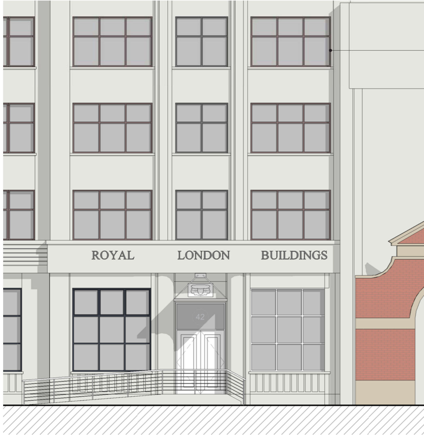
▲ Existing facade with white framed window to the right of the entrance, different from the rest of the ground floor windows
