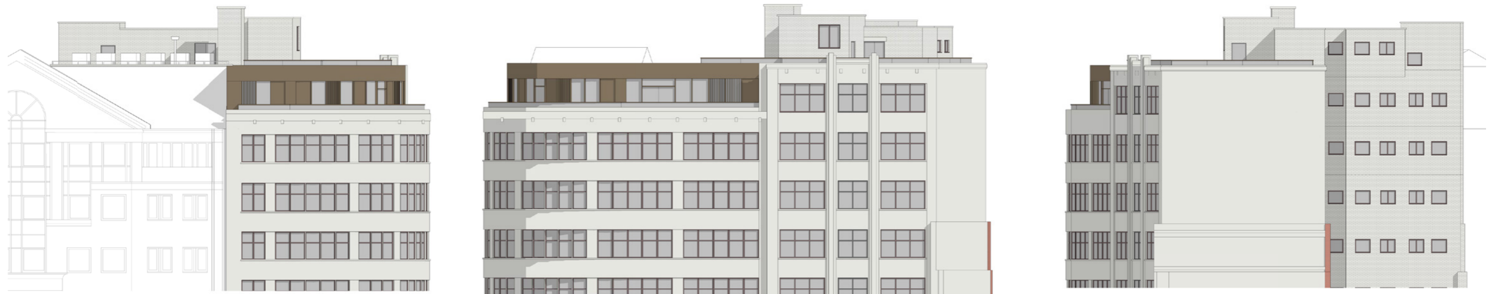
▲ Proposed East, North and West elevation showing the extension in powder coated metal to compliment the existing materiality
