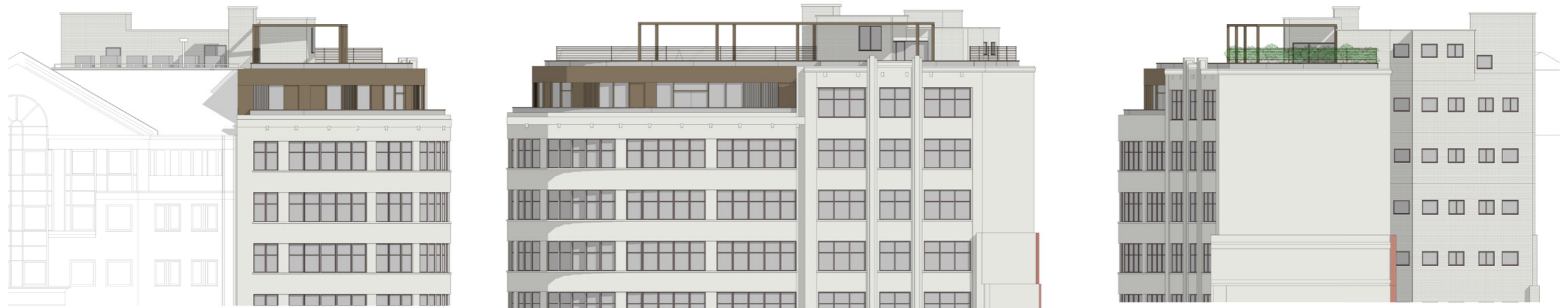
▲ Proposed East, North and West elevation showing the extension in powder coated metal to compliment the existing materiality
