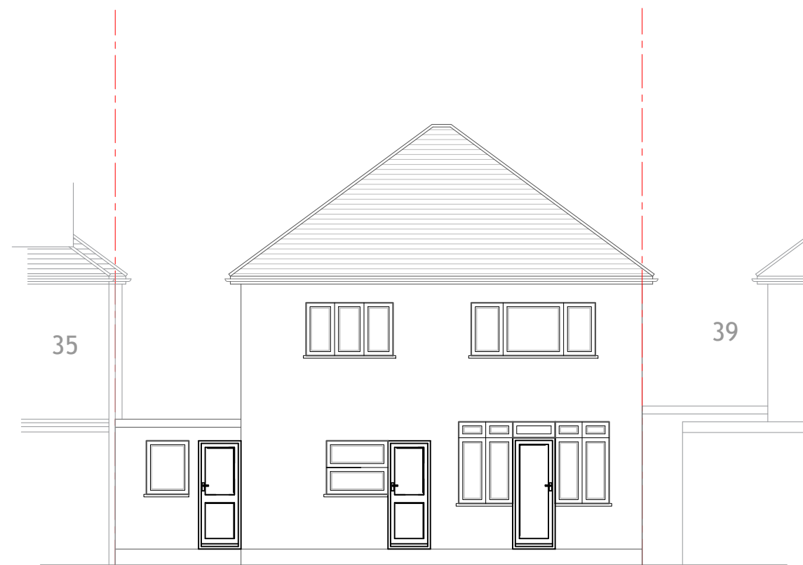
EXISTING REAR ELEVATION
