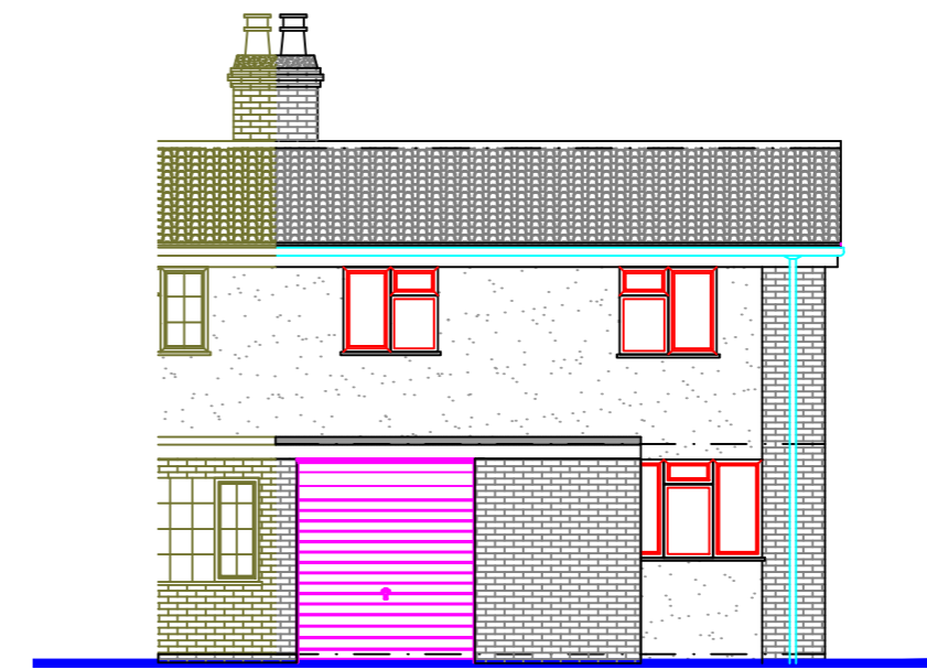
EXISTING SOUTH ELEVATION... Scale 1:100
