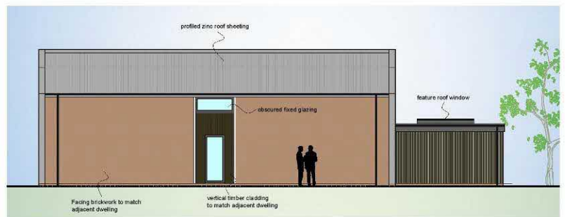
Proposed South Elevation (1:100)
