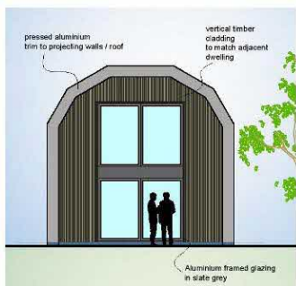
Proposed West Elevation (1:100)
