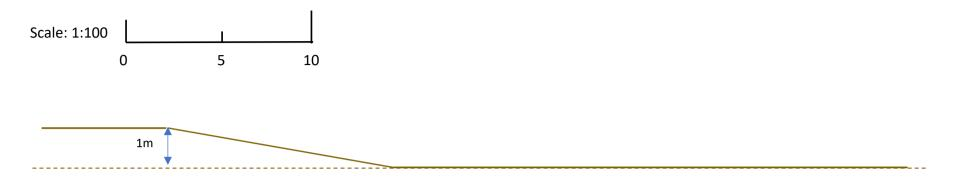
The ground slopes down from the north west corner for about 6m along the north boundary, to a level of c. 1m lower.
