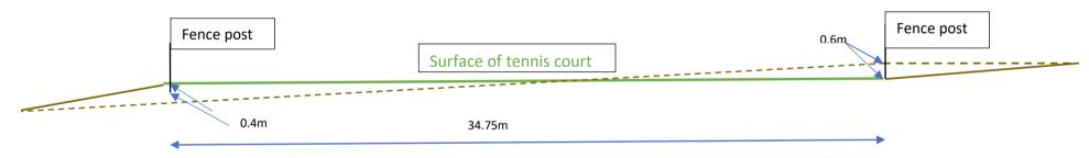
The groundworks will level the area such that the soil is taken from the north western corner and moved to the south eastern corner, creating a level which will be c.40cm above the level of the garden and 60cm below the level of the boundary.
