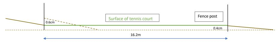
The groundworks will level the area such that the soil is taken from the north western corner and moved to the south eastern corner, creating a level which will be c.40cm above the level of the garden and 60cm below the level of the boundary.
