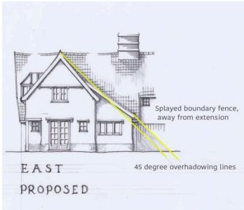
Due to the historical importance of the existing staircase, this negates the need for a new staircase (as shown initially), however access to the extension would be via the flat roof dormer. Combined with the narrowing of the gable and a traditional pitch roof, this allows the buildings ridge (overshadowing point) to be moved as far South West as possible.
