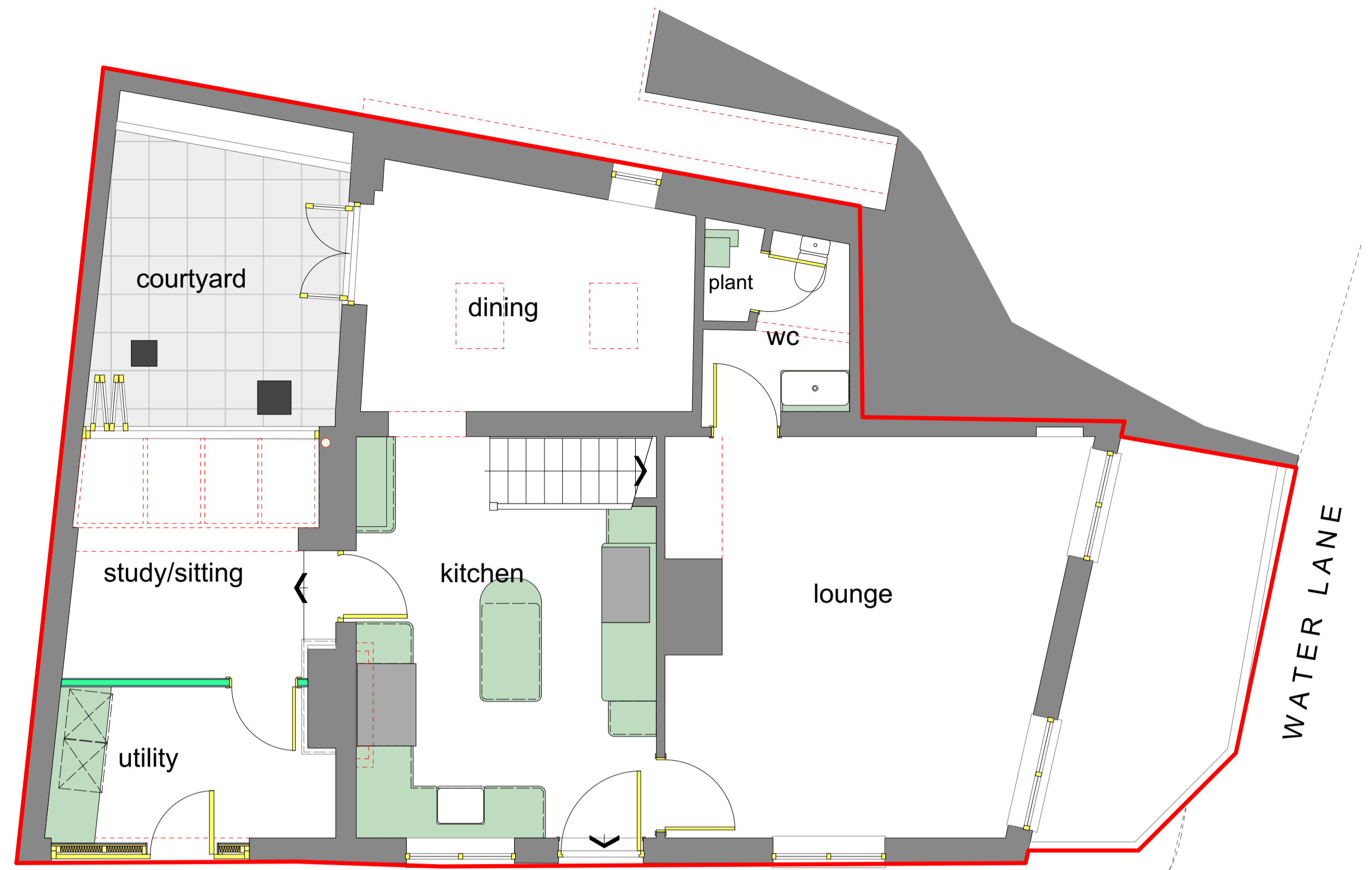
GROUND FLOOR PLAN Scale 1:50
