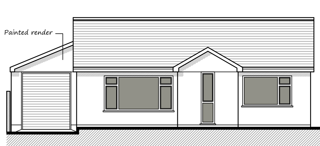
South West Elevation
