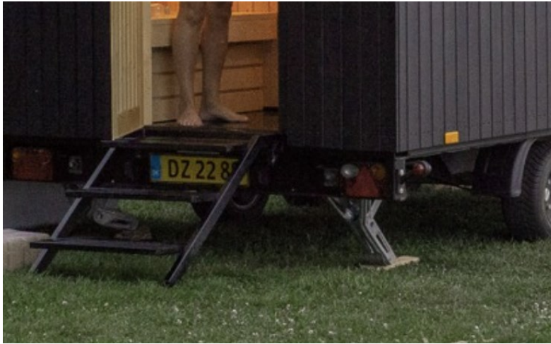
Figure 13: Example of flat bed trailer and retractable stairs
