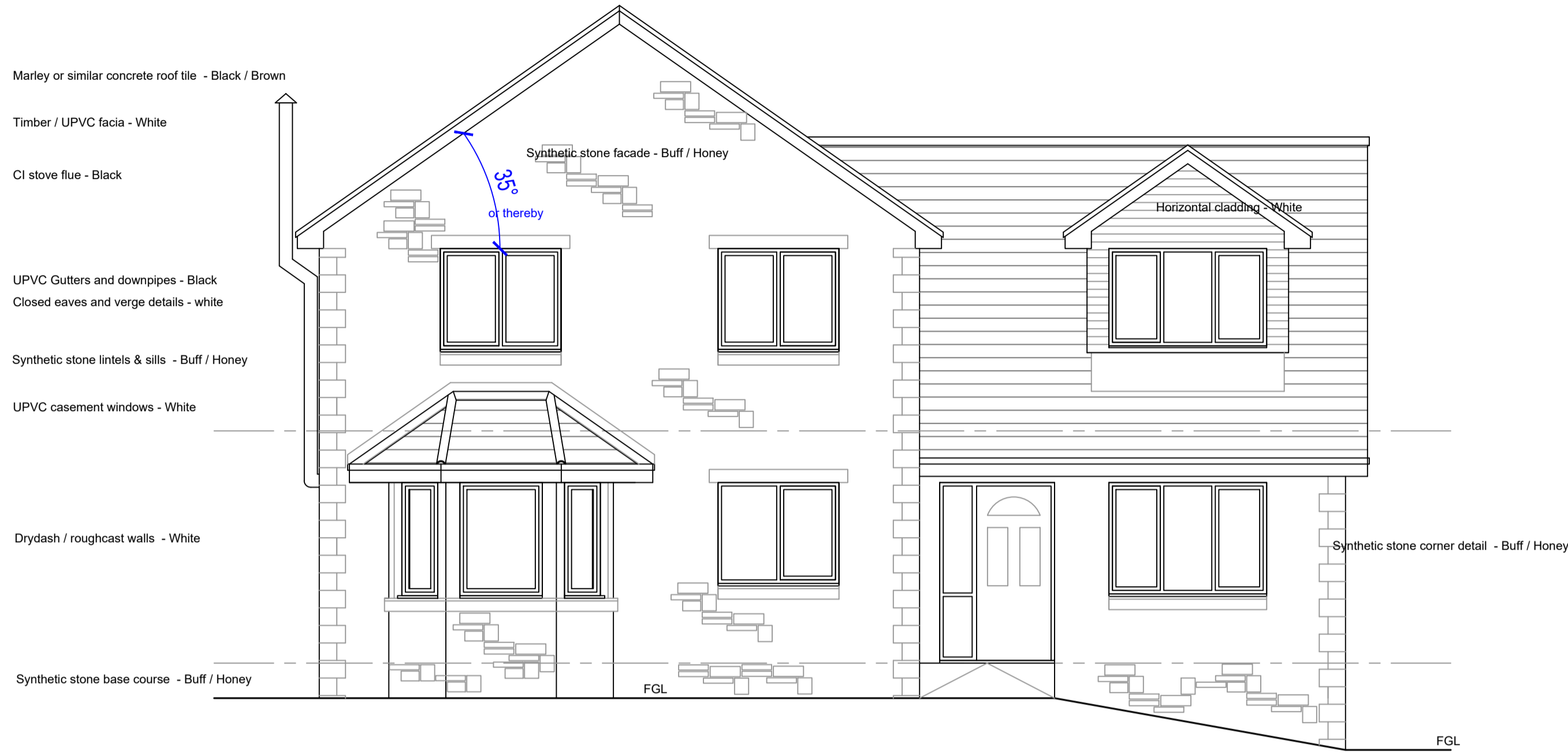
Front Elevation (West) as Existing 1:50
