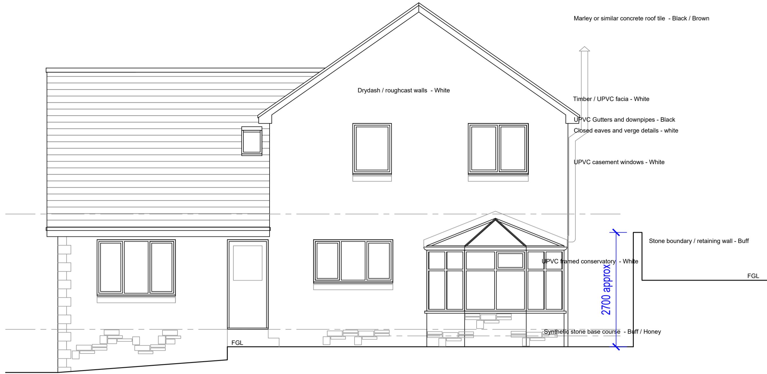
Rear Elevation (East) as Existing 1:50
