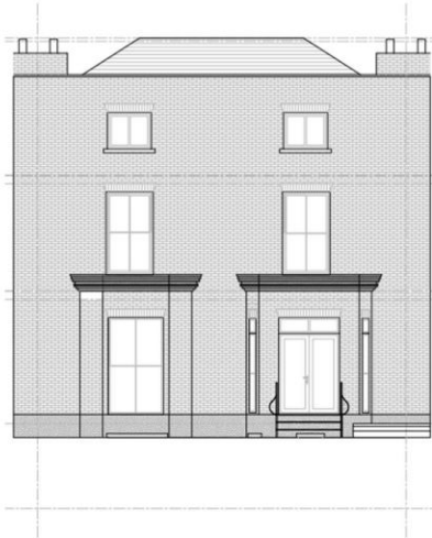
EXISTING REAR (SOUTH) ELEVATION 1:50@A1
