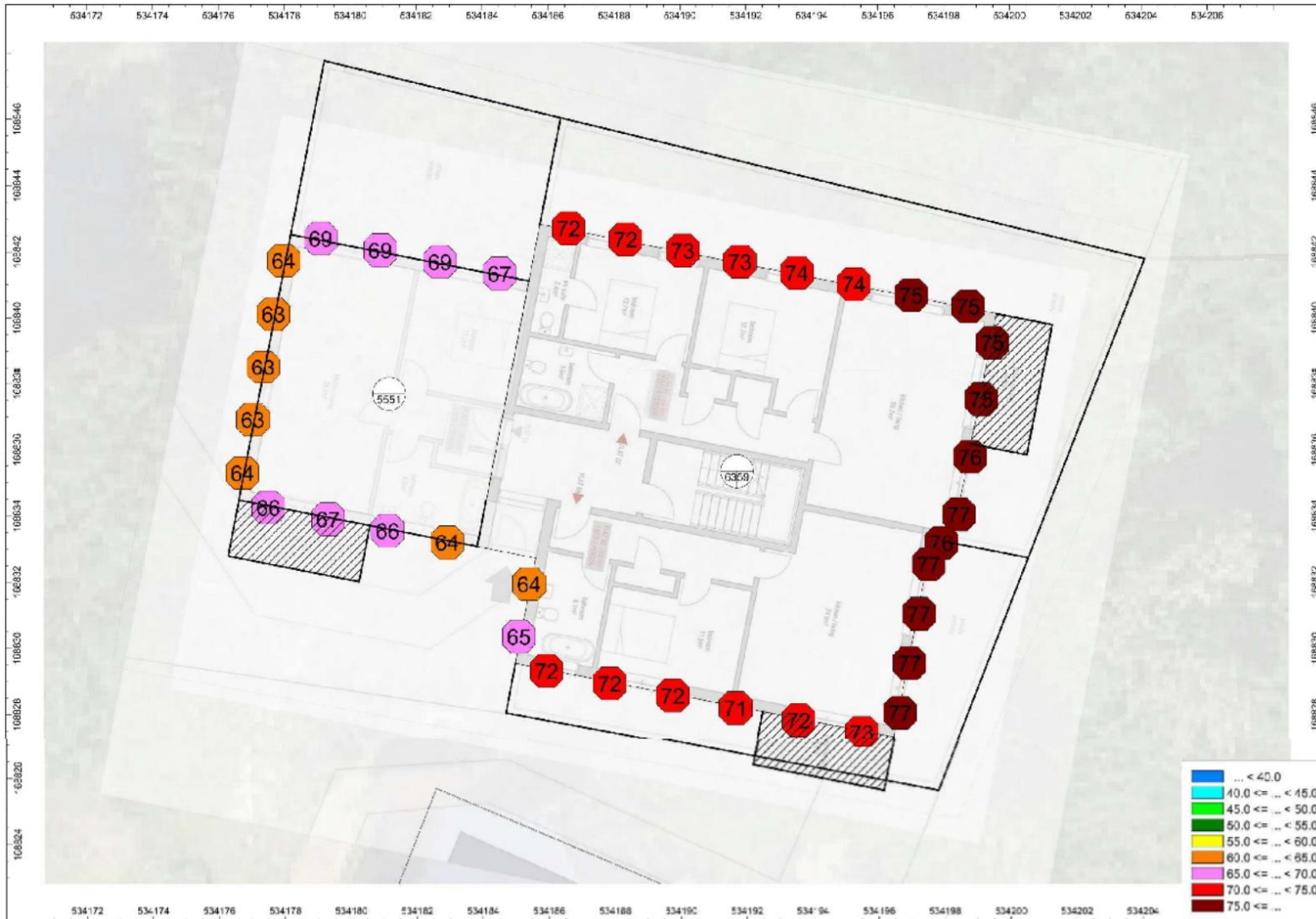
Figure D.9 – Proposed development - Predicted 10 th highest per night dB L AFmax exposure levels – Night-time (23:00 – 07:00)
