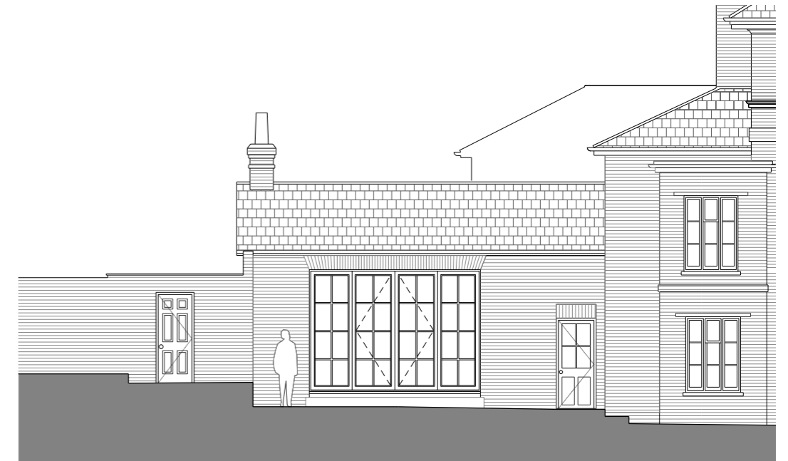
Proposed south-west elevation including timber frame double French doors to sit within the area of non-original and heavily altered brickwork, and including soldier course brickwork.
