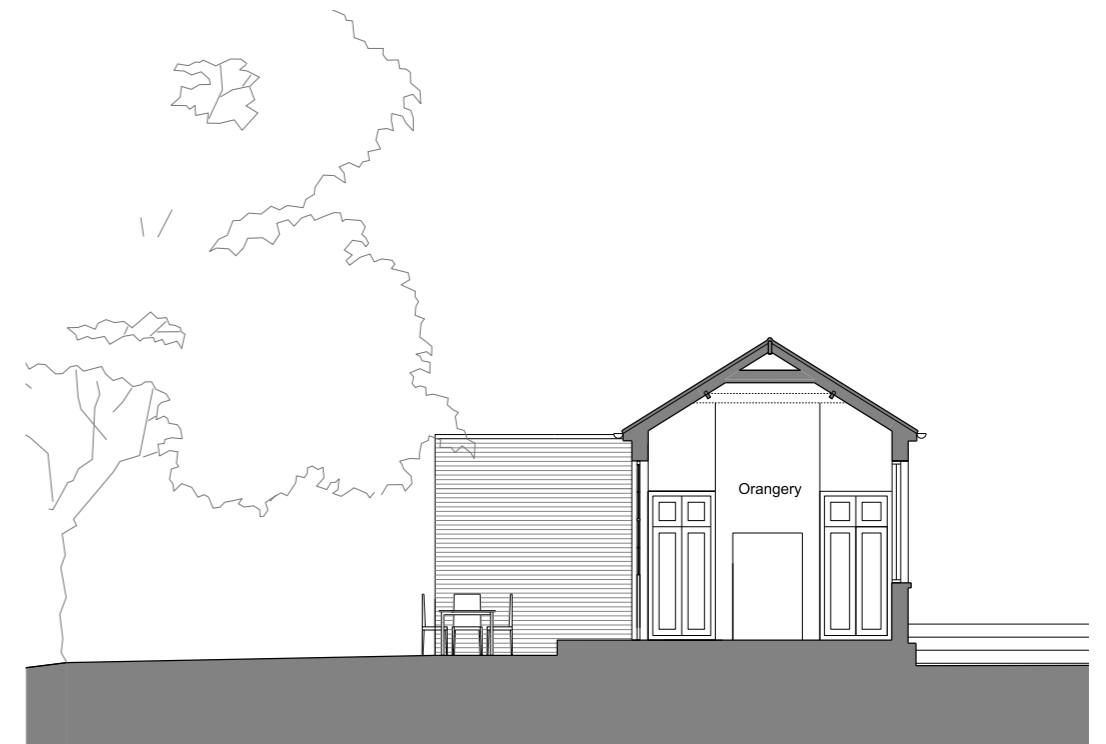
Section through orangery showing removal of non-original ceiling and reinstated room proportions
