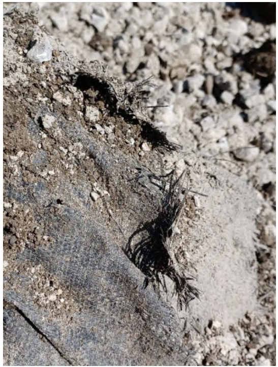
TP04 Spoil heap- close up of geotextile layer.
