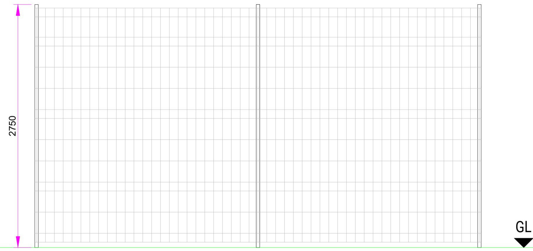
WELDED MESH FENCE ELEVATION
