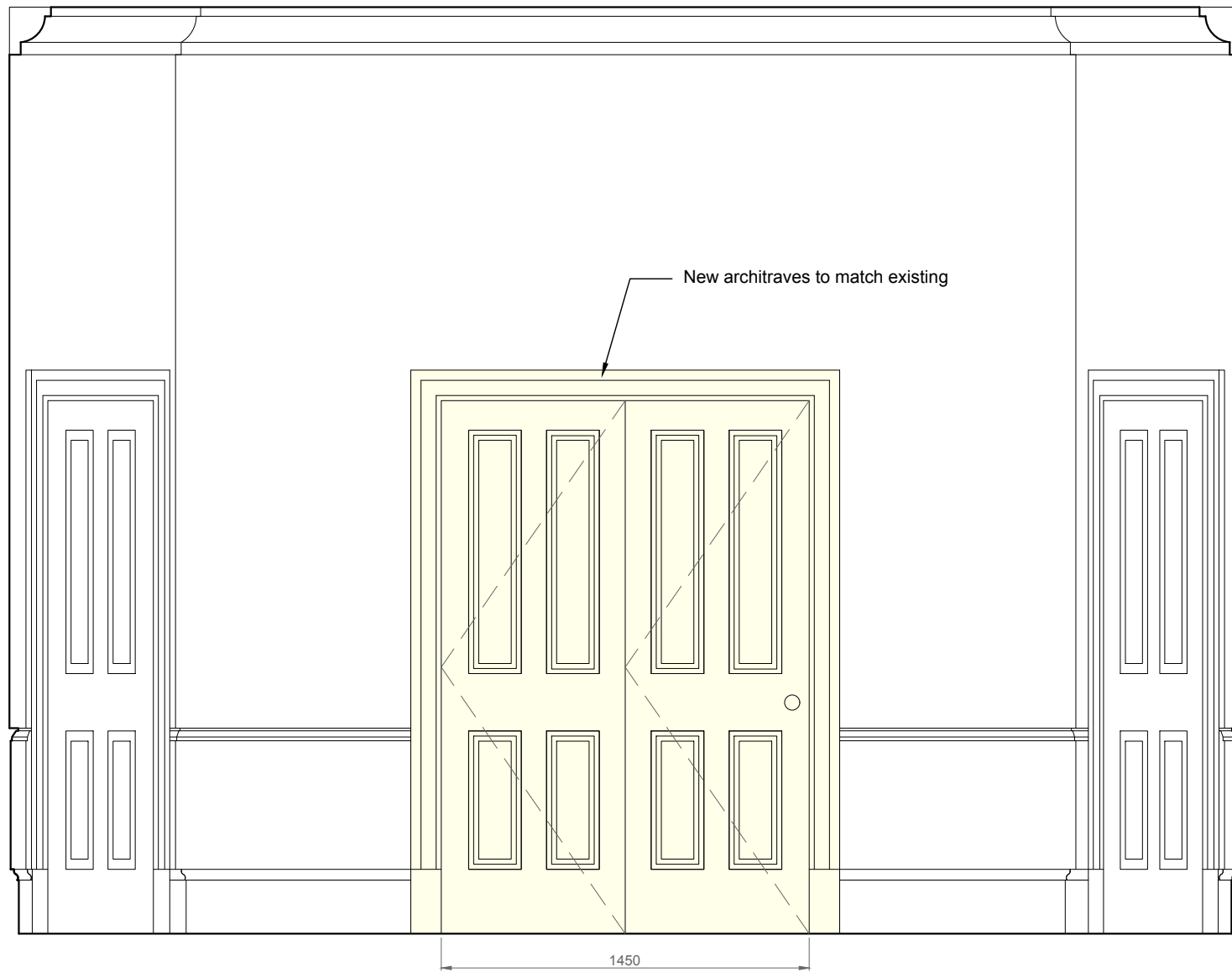
Proposed new ground floor door. View from drawing room scale 1:25
