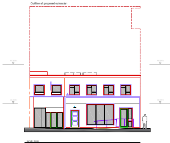
Existing Front elevation - North Scale 1:100 @ A1
