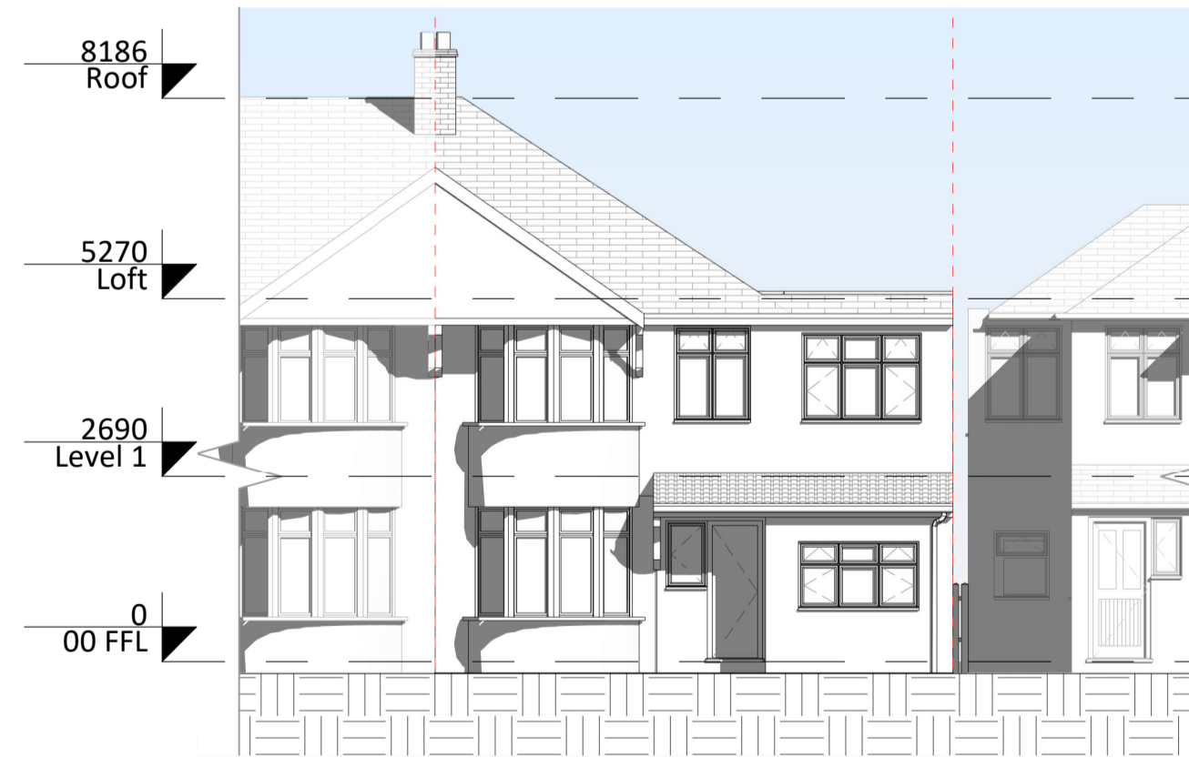
5 Existing Front Elevation 1 : 100
