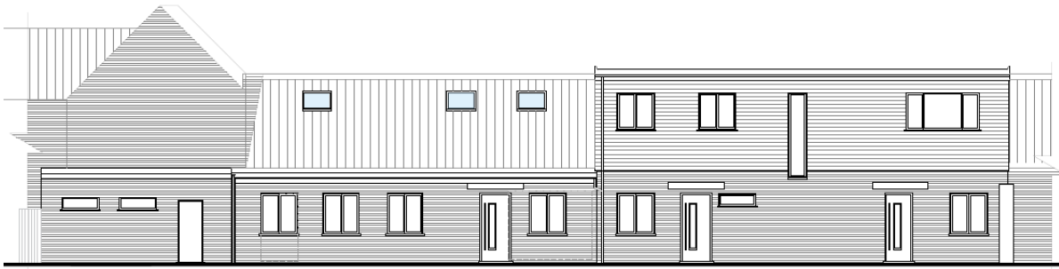
① Proposed front elevation 1:100
