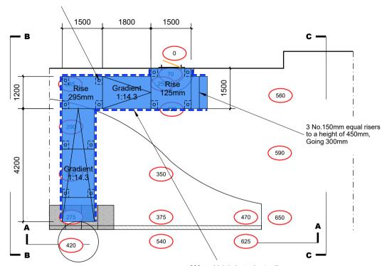
900mm high balustrades to all ramps Handrails comprise vinyl covered 40 x 5mm flat steel bar at a height of 900mm above stair pitch line. No opening in balustrade permits the passage of a sphere of diameter 100mm.
