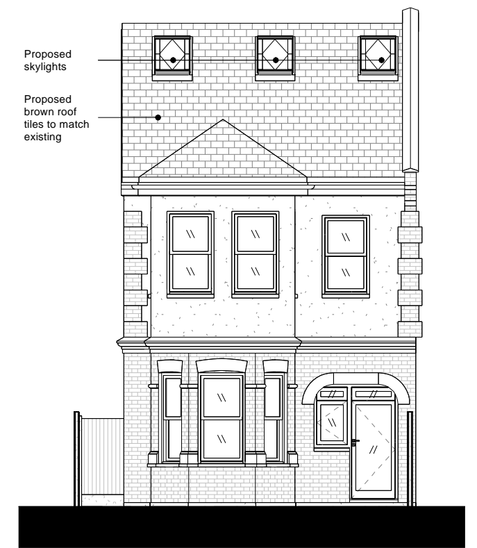
Figure 034 - Proposed Front Elevation - West
