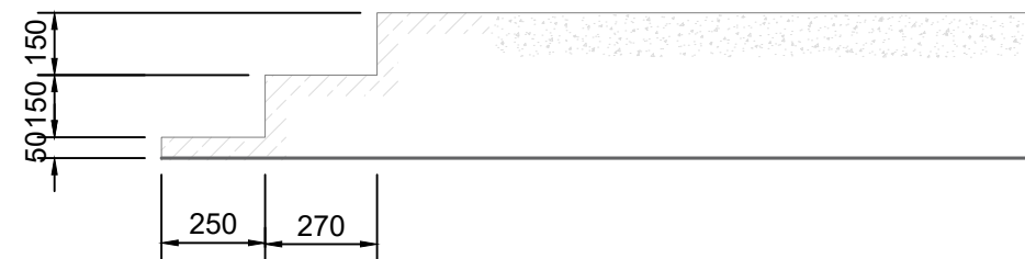
A-A Existing Staircase Section 1:20
