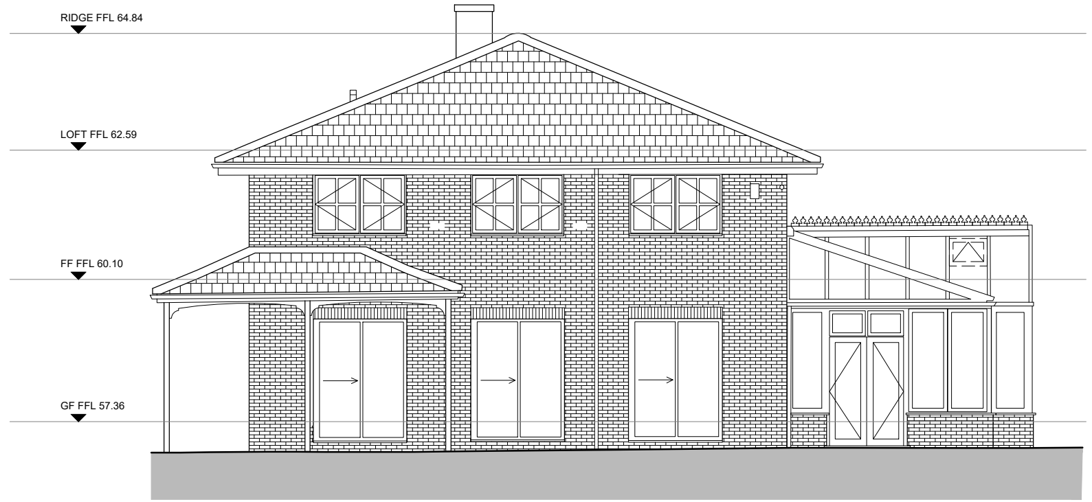
NORTH ELEVATION AS EXISTING (FRONT)
