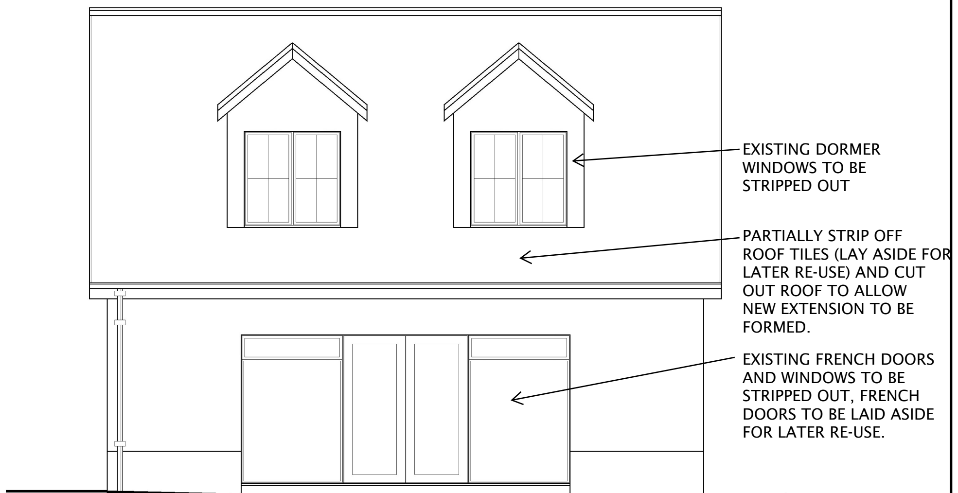
EXISTING FRONT ELEVATION SCALE 1:50
