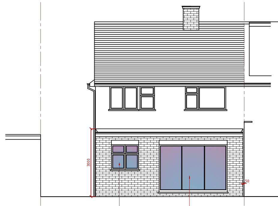
WINDOW TO MATCH EXISTING DWELLING BI-FOLD DOORS TO SPECIALIST DETAILS PROPOSED REAR ELEVATION
