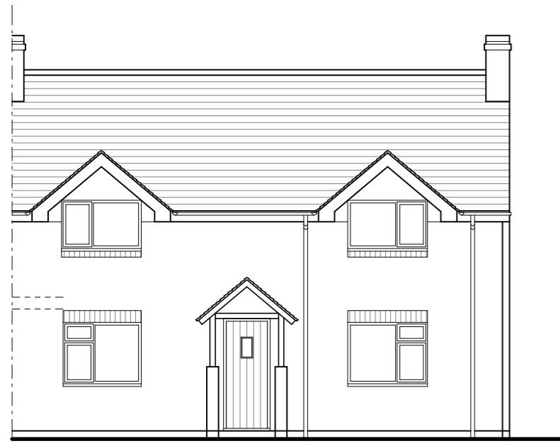
FRONT ELEVATION AS PROPOSED Scale 1:100 Facing Brick and Roof Tiles to match existing dwelling
