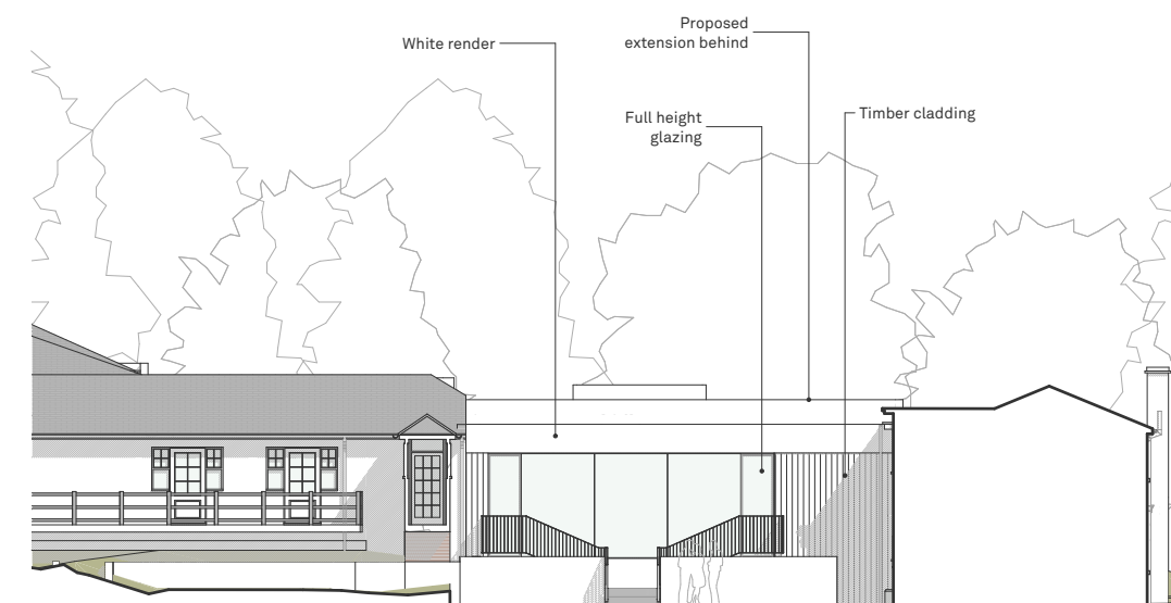
Proposed courtyard facing elevation
