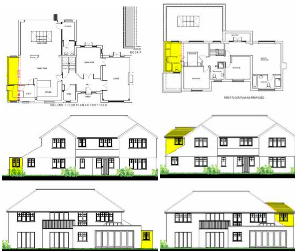
Figure 3 Left: Extract of Elevations and Floorplans on application 23/0467/CES, showing single storey side extension to remain unbuilt; Right: Extract of Proposed First Floor Plan and Elevations for this Proposal, highlighted to show relevant areas of built form.
