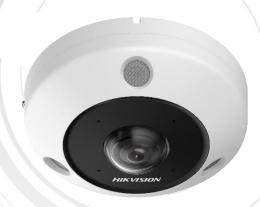
DS-2CD63C5G1-IVS is a fisheye network camera capable of providing a 360-degree panoramic image of its scene. The progressive scan CMOS sensor provides high-resolution images of up to 3504 × 3504. Up to 20 live view display modes, designed for 3 mount types, meet various user preferences. Three independently controlled IR lights offer a range of 15 m and provide good vision in low or even zero-light environment.
