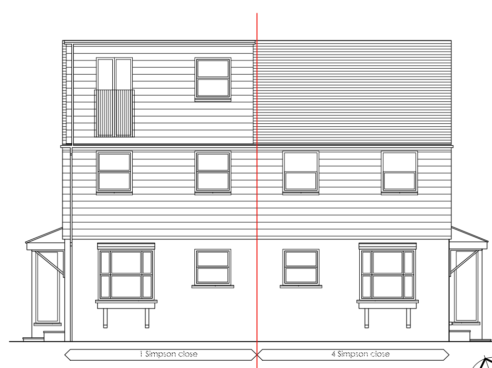
EXISTING SIDE ELEVATION (SOUTH) 1:100
