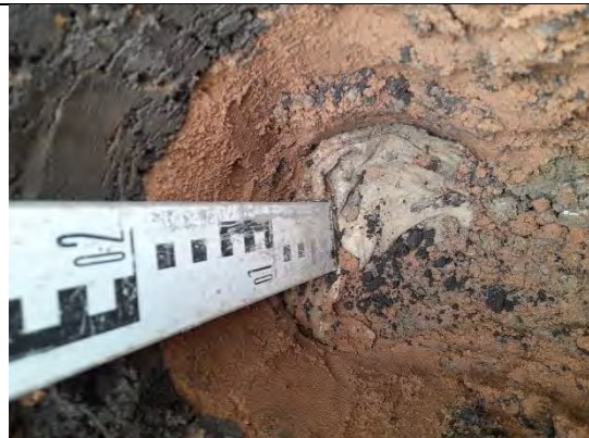
Photograph 169: View of soil within cover system and geotextile at base in rear (S) of Plot 62.
