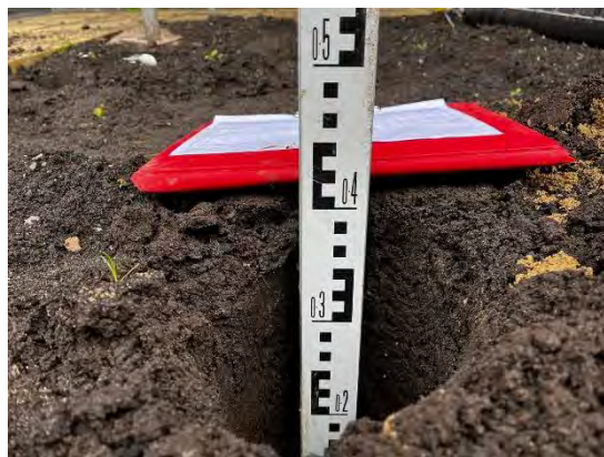
Photograph 104: View of depth of soil within the front garden of Plot 51.
