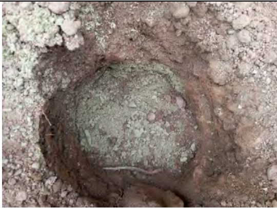
Photograph 27: View of soil within cover system and geotextile at base in rear (N) of Plot 39.
