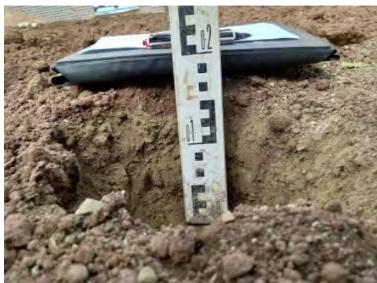
Photograph 32: View of depth of soil within the rear (N) garden of Plot 40.
