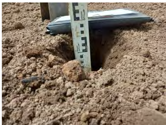
Photograph 50: View of depth of soil within the rear (N) garden of Plot 42.
