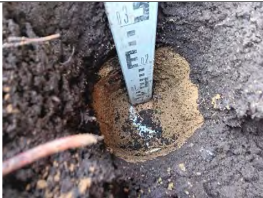
Photograph 69: View of soil within cover system and geotextile at base in front of Plot 45.
