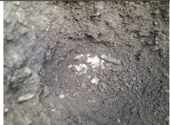
Photograph 30: View of soil within cover system and geotextile at base in front of Plot 40.
