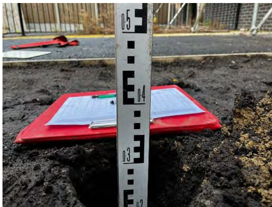
Photograph 98: View of depth of soil within the front garden of Plot 50.
