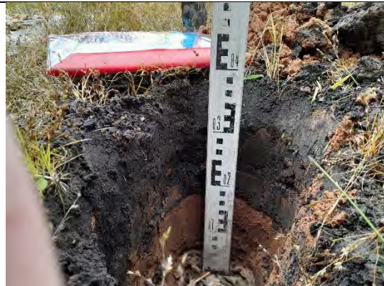
Photograph 168: View of depth of soil within the rear garden (S) of Plot 62
