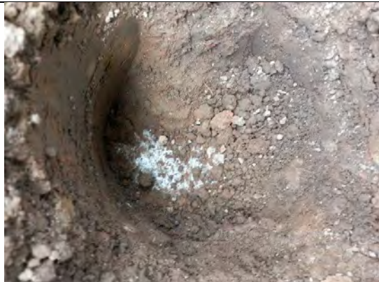
Photograph 51: View of soil within cover system and geotextile at base in rear (N) of Plot 42.
