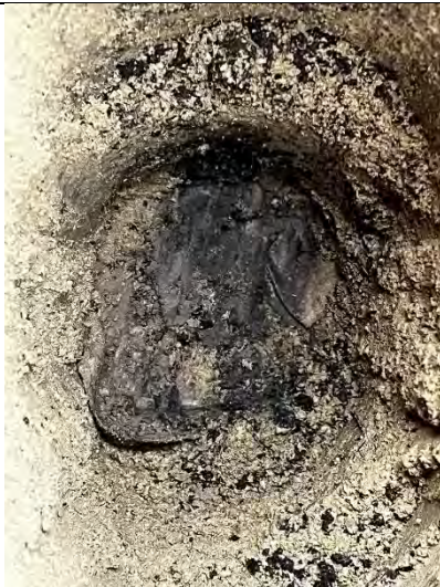
Photograph 154: View of soil within cover system and geotextile at base in rear of Plot 60.
