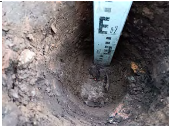
Photograph 9: View of soil within cover system and geotextile at base in rear (S) of Plot 37.
