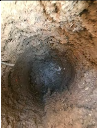
Photograph 172: View of soil within cover system and geotextile at base of shared soft landscaping A1.
