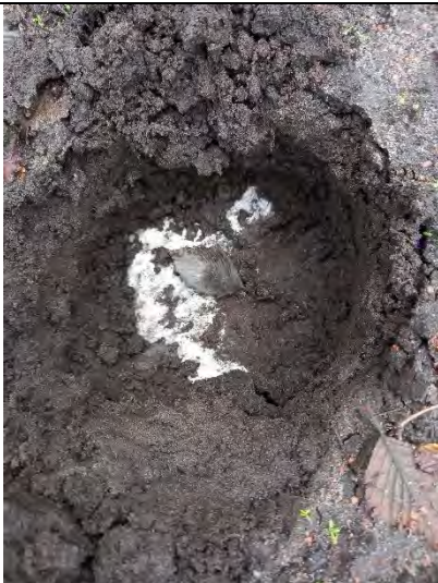
Photograph 183: View of soil within cover system and geotextile at base of shared soft landscaping B2.
