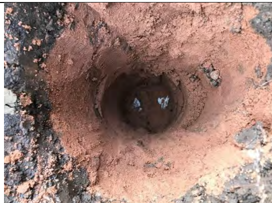
Photograph 160: View of soil within cover system and geotextile at base in rear of Plot 61.
