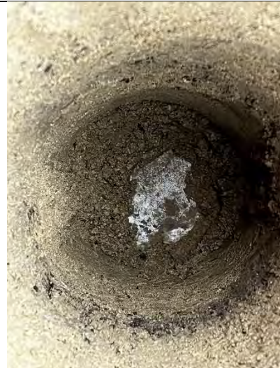
Photograph 151: View of soil within cover system and geotextile at base in rear of Plot 59.
