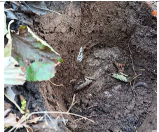
Photograph 18: View of soil within cover system and geotextile at base in rear (S) of Plot 38.
