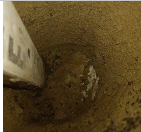
Photograph 133: View of soil within cover system and geotextile at base in rear of Plot 56.
