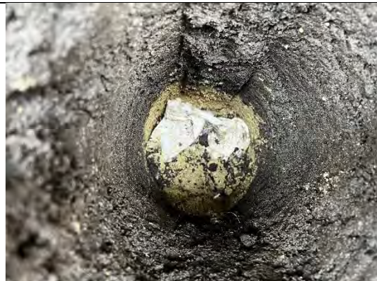
Photograph 105: View of soil within cover system and geotextile at base in front of Plot 51.
