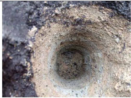
Photograph 90: View of soil within cover system and geotextile at base in rear of Plot 48.
