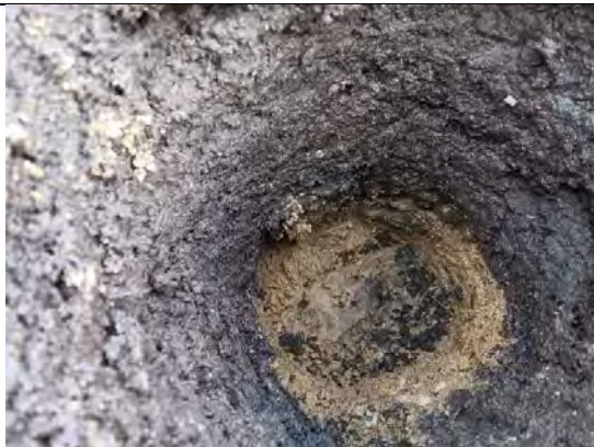
Photograph 75: View of soil within cover system and geotextile at base in front of Plot 46.
