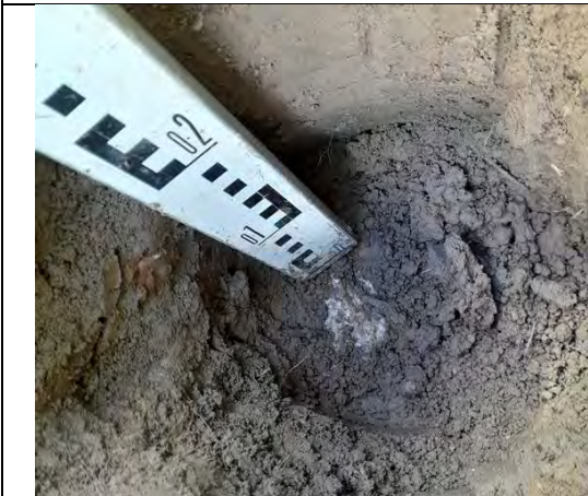
Photograph 15: View of soil within cover system and geotextile at base in rear (N) of Plot 38.
