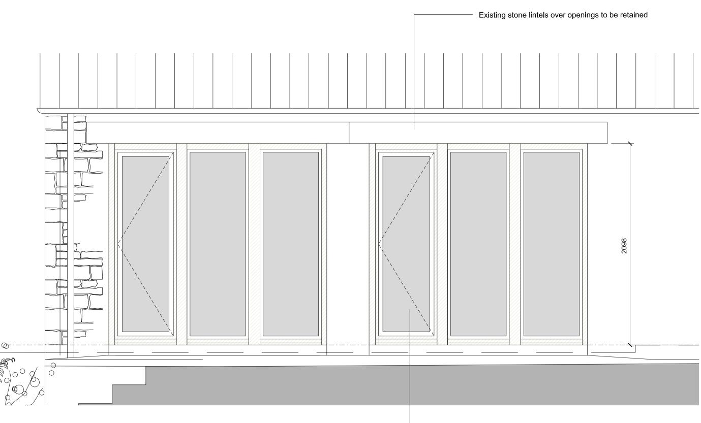
Proposed timber windows to fill existing garage door openings.
