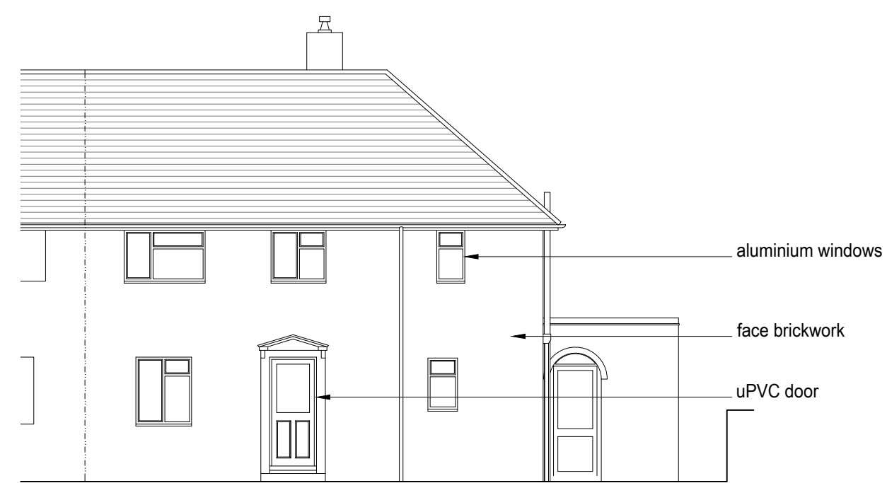
Existing Front Elevation 1:100
