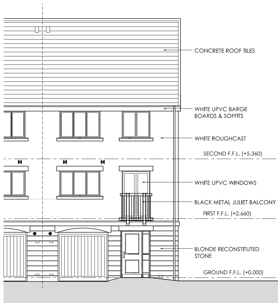
EXISTING EAST ELEVATION
