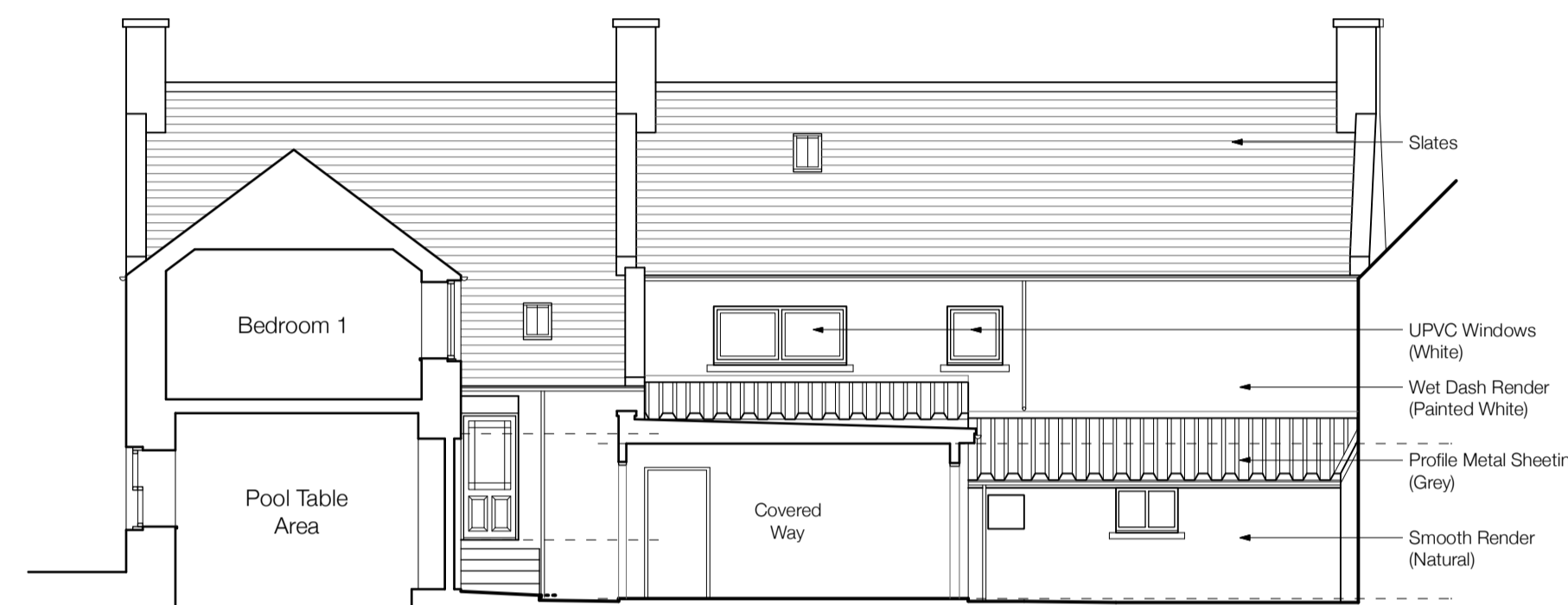
West Sectional Elevation 1:100
