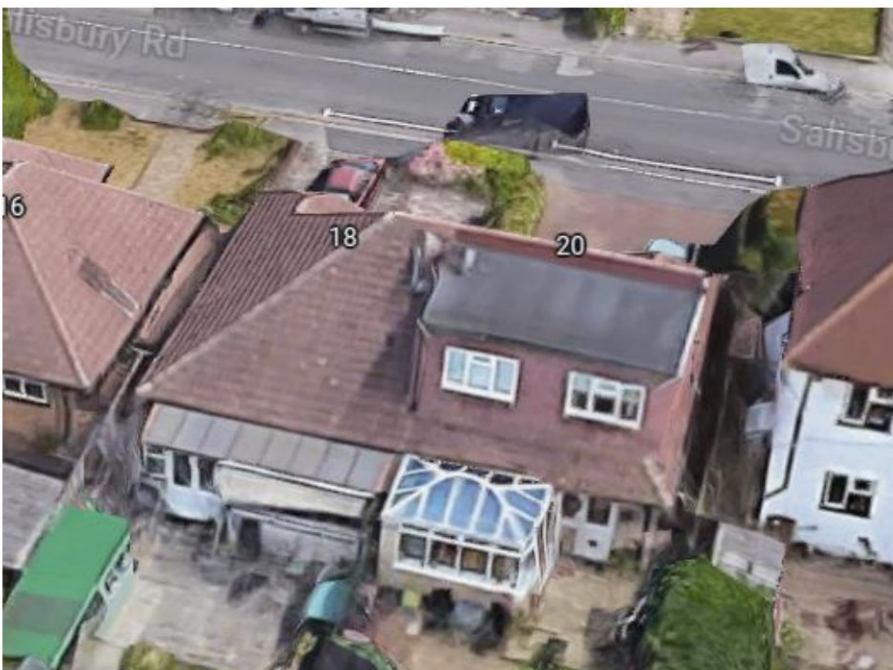
Aerial view of 20 Salisbury Road showing rear dormer on a hip to gable roof conversion.
